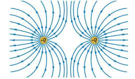
Figure 19.27 The electric field near two equal positive charges is directed away from each of the charges.
