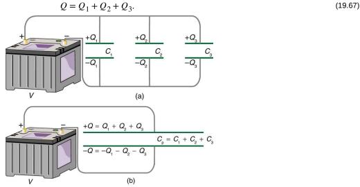
Figure 19.22 (a) Capacitors in parallel. Each is connected directly to the voltage source just as if it were all alone, and so the total capacitance in parallel is just the sum of the individual capacitances. (b) The equivalent capacitor has a larger plate area and can therefore hold more charge than the individual capacitors.
