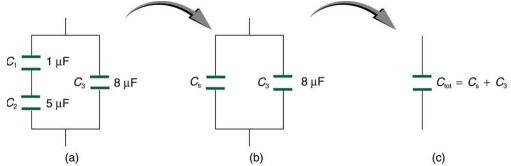
Figure 19.23 (a) This circuit contains both series and parallel connections of capacitors. See Example 19.10 for the calculation of the overall capacitance of the circuit. (b)  $C_1$  and  $C_2$  are in series; their equivalent capacitance  $C_S$  is less than either of them. (c) Note that  $C_S$  is in parallel with  $C_S$ . The total capacitance is, thus, the sum of  $C_S$  and  $C_S$ .
