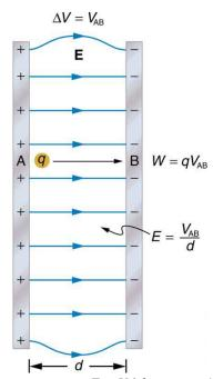
Figure 19.5 The relationship between V and E for parallel conducting plates is E = V/d. (Note that  $\Delta V = V_{AB}$  in magnitude. For a charge that is moved from plate A at higher potential to plate B at lower potential, a minus sign needs to be included as follows:  $-\Delta V = V_A - V_B = V_{AB}$ . See the text for details.)
