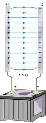
Figure 19.14 Electric field lines in this parallel plate capacitor, as always, start on positive charges and end on negative charges. Since the electric field strength is proportional to the density of field lines, it is also proportional to the amount of charge on the capacitor.
