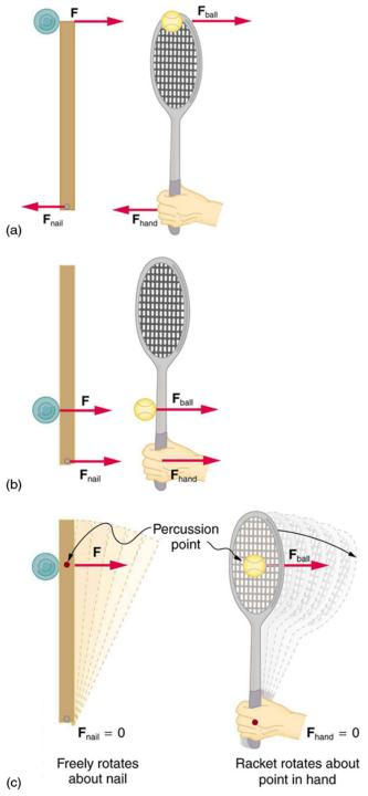
Figure 10.27 A disk hitting a stick is compared to a tennis ball being hit by a racquet. (a) When the ball strikes the racquet near the end, a backward force is exerted on the hand. (b) When the racquet is struck much farther down, a forward force is exerted on the hand. (c) When the racquet is struck at the percussion point, no force is delivered to the hand.
