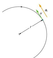
Figure 10.4 In circular motion, linear acceleration a, occurs as the magnitude of the velocity changes: a is tangent to the motion. In the context of circular motion, linear acceleration is also called tangential acceleration  $a_{1}$ .
