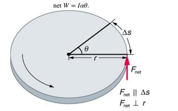
Figure 10.15 The net force on this disk is kept perpendicular to its radius as the force causes the disk to rotate. The net work done is thus (net F) $\Delta s$ . The net work goes into rotational kinetic energy.
