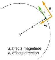
Figure 10.5 Centripetal acceleration  $a_c$  occurs as the direction of velocity changes; it is perpendicular to the circular motion. Centripetal and tangential acceleration are thus perpendicular to each other.
