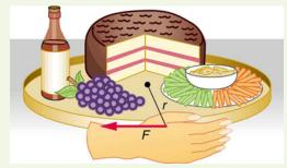
Figure 10.21 A partygoer exerts a torque on a lazy Susan to make it rotate. The equation net  $\tau = \frac{\Delta L}{\Delta t}$  gives the relationship between torque and the angular momentum produced.
