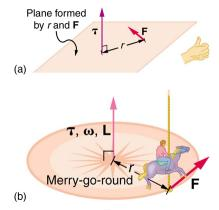
Figure 10.29 In figure (a), the torque is perpendicular to the plane formed by r and  $\mathbf{F}$  and is the direction your right thumb would point to if you curled your fingers in the direction of  $\mathbf{F}$ . Figure (b) shows that the direction of the torque is the same as that of the angular momentum it produces.
