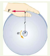
Figure 10.17 A large grindstone is given a spin by a person grasping its outer edge.
