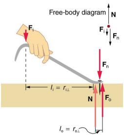
Figure 9.23 A nail puller is a lever with a large mechanical advantage. The external forces on the nail puller are represented by solid arrows. The force that the nail puller applies to the nail ( $\mathbf{F}_0$ ) is not a force on the nail puller. The reaction force the nail exerts back on the puller ( $\mathbf{F}_n$ ) is an external force and is equal and opposite to  $\mathbf{F}_0$ . The perpendicular lever arms of the input and output forces are  $\,l_{i}\,$  and  $\,l_{0}\,$  .
