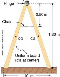
Figure 9.35 A sandwich board advertising sign demonstrates tension.
