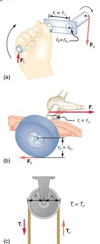
Figure 9.25 (a) A crank is a type of lever that can be rotated 360° about its pivot. Cranks are usually designed to have a large MA. (b) A simplified automobile axle drives a wheel, which has a much larger diameter than the axle. The MA is less than 1. (c) An ordinary pulley is used to lift a heavy load. The pulley changes the direction of the force T exerted by the cord without changing its magnitude. Hence, this machine has an MA of 1.
