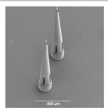
Figure 1.24: SEM image of micro-needles (Source: www.belasnet.be<sup>9</sup>).
