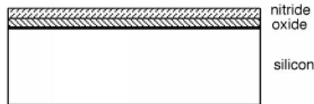
**Figure 4.18:** Initial wafer configuration.
